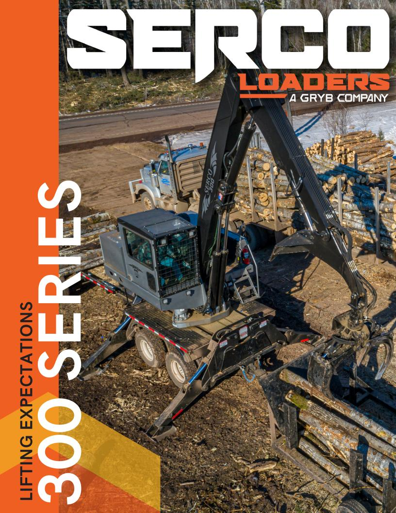
The SERCO 300 is available in truck mount, self propelled carrier, or stationary electric applications. With a wide variety of options and on-demand hydraulics, this loader is exceptional for applications in the forestry, scrap, or industrial material handling industries.
